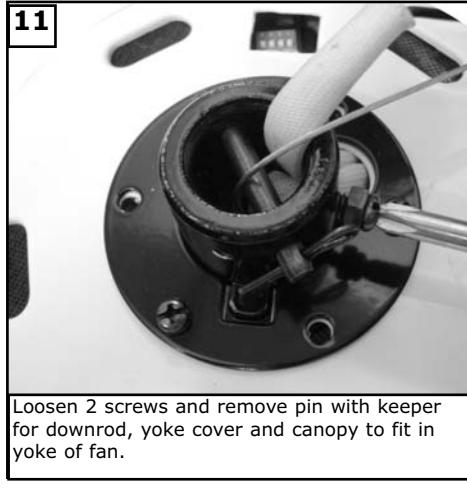
Loosen 2 screws and remove pin with keeper for downrod, yoke cover and canopy to fit in yoke of fan.
